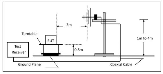
(c) For radiated emissions above 1000MHz
