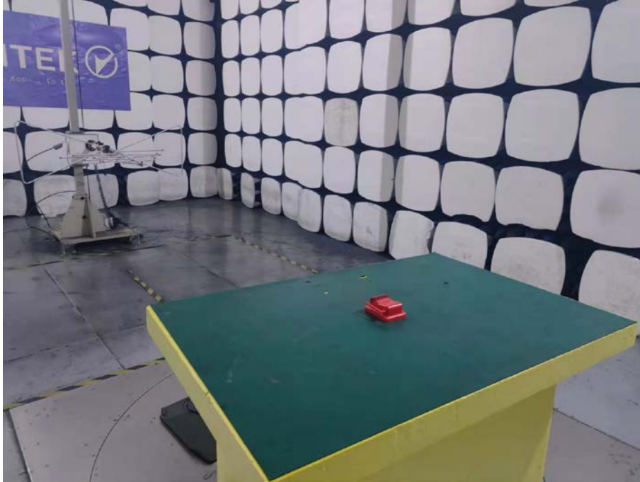
Spurious Emission Test Setup (Above 1GHz)
