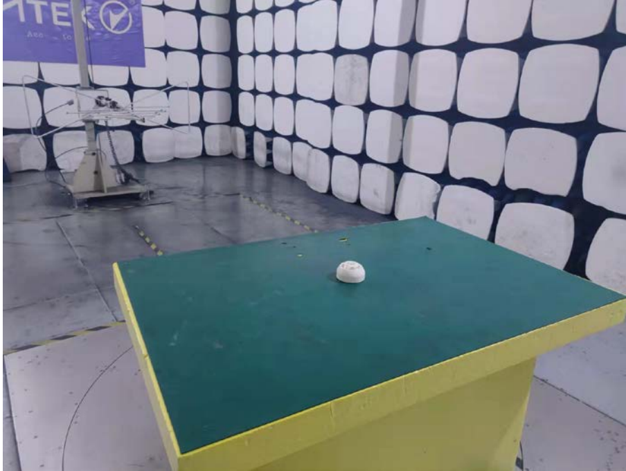
Spurious Emission Test Setup (Above 1GHz)
