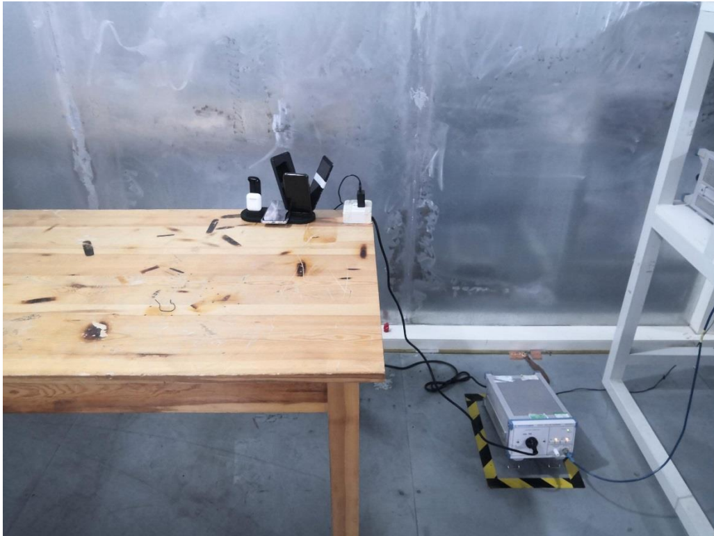
Conducted Emission-AC adapter charge mode
