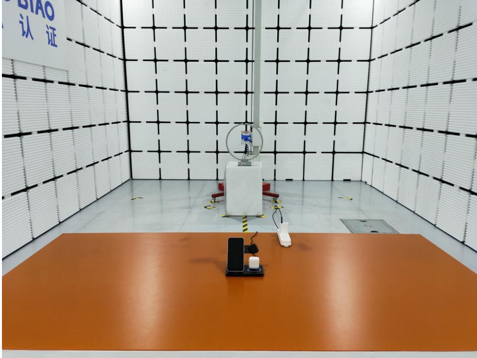
Radiated Emission Above 30MHz
