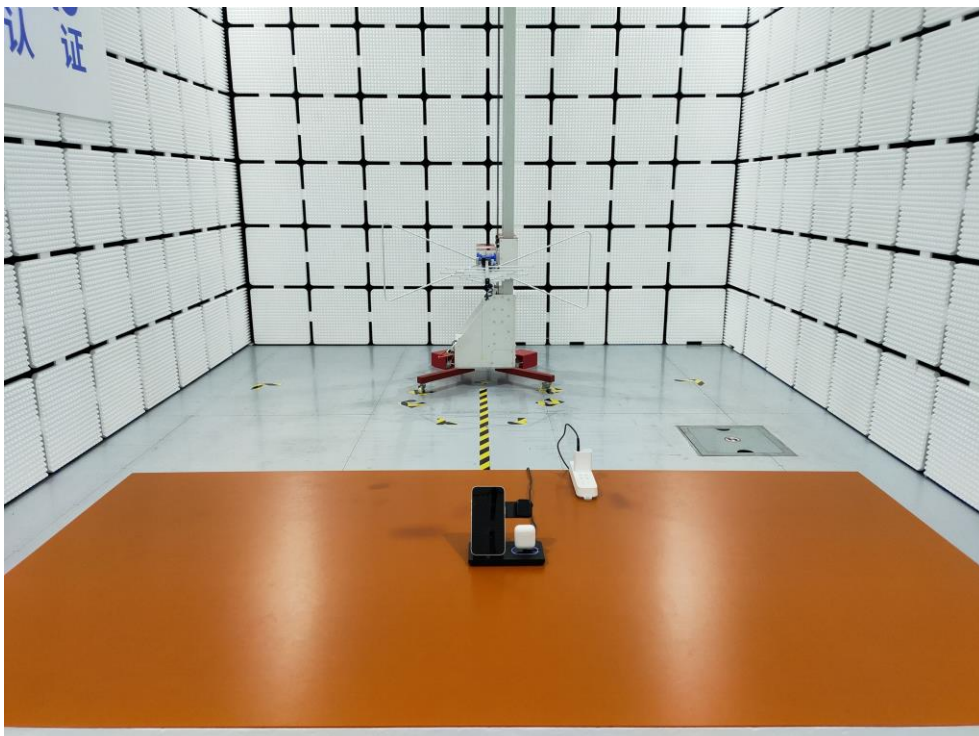
Radiated Emission Above 30MHz
