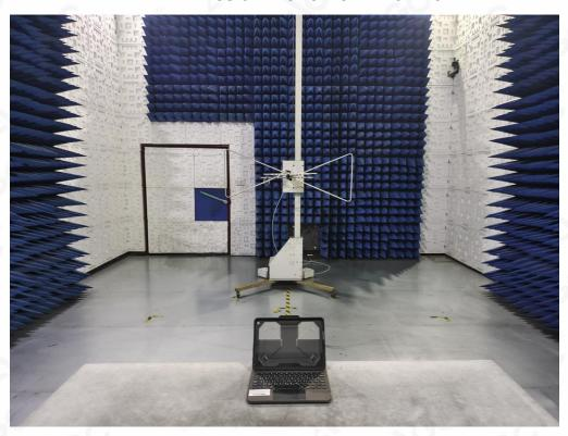
RADIATED EMISSION TEST SETUP ABOVE 1GHz
