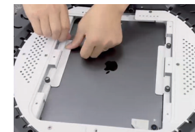
Step 11: Fix your iPad on Panel with Fixed Plate
