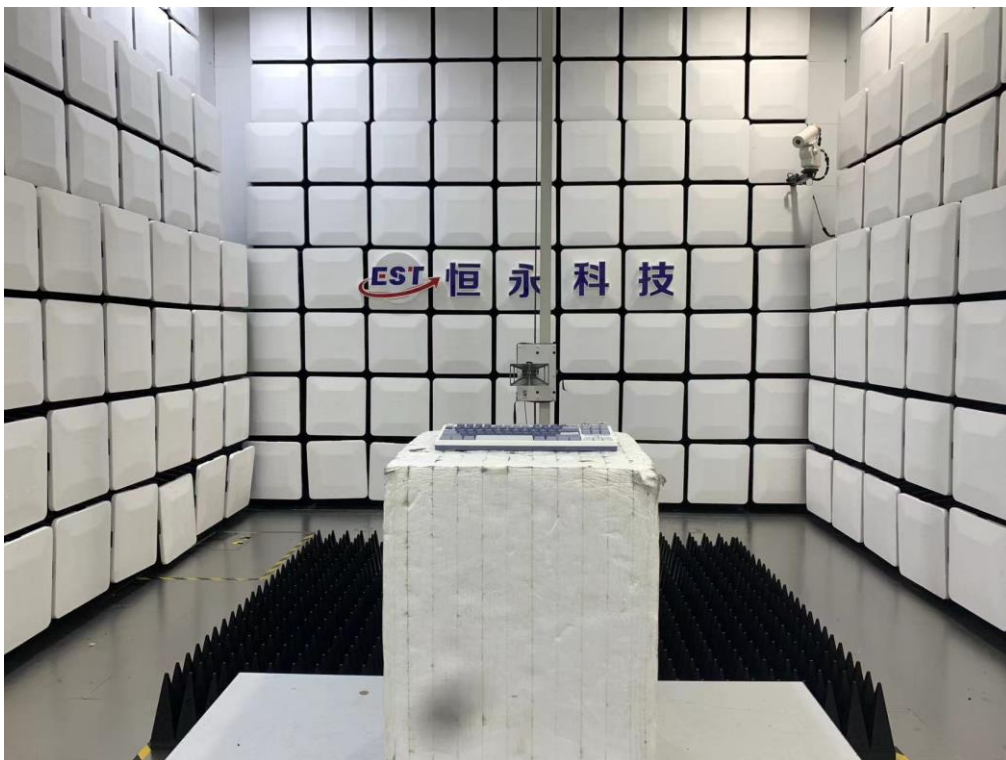
Radiated emission test: Above 1GHz
