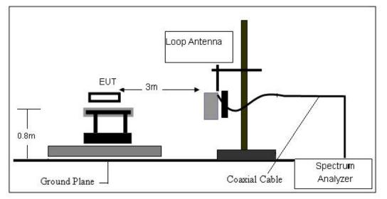
(B) Radiated Emission Test-Up Frequency 30MHz~1GHz
