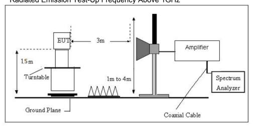
Radiated Emission Test-Up Frequency Above 1GHz
