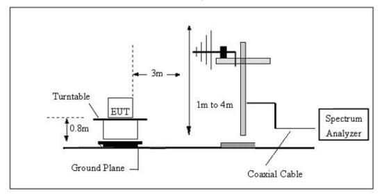
(C) Radiated Emission Test-Up Frequency Above 1GHz
