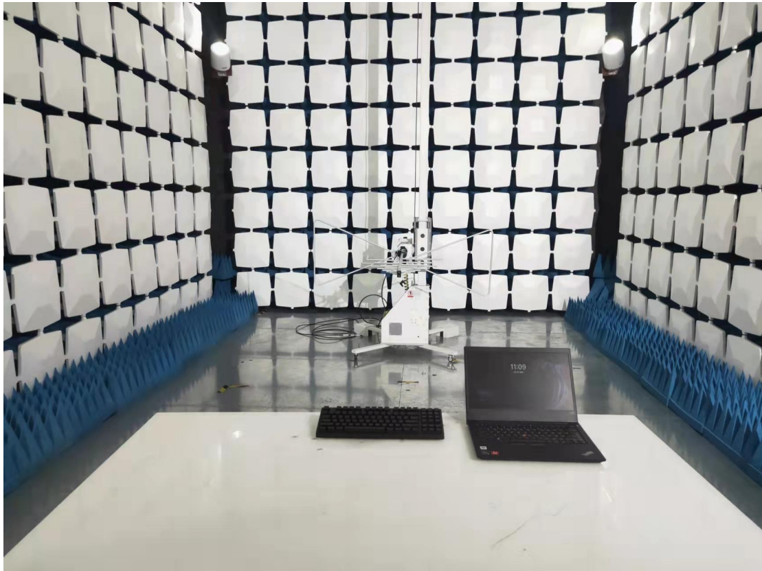
Above 1GHz for radiated emission test setup
