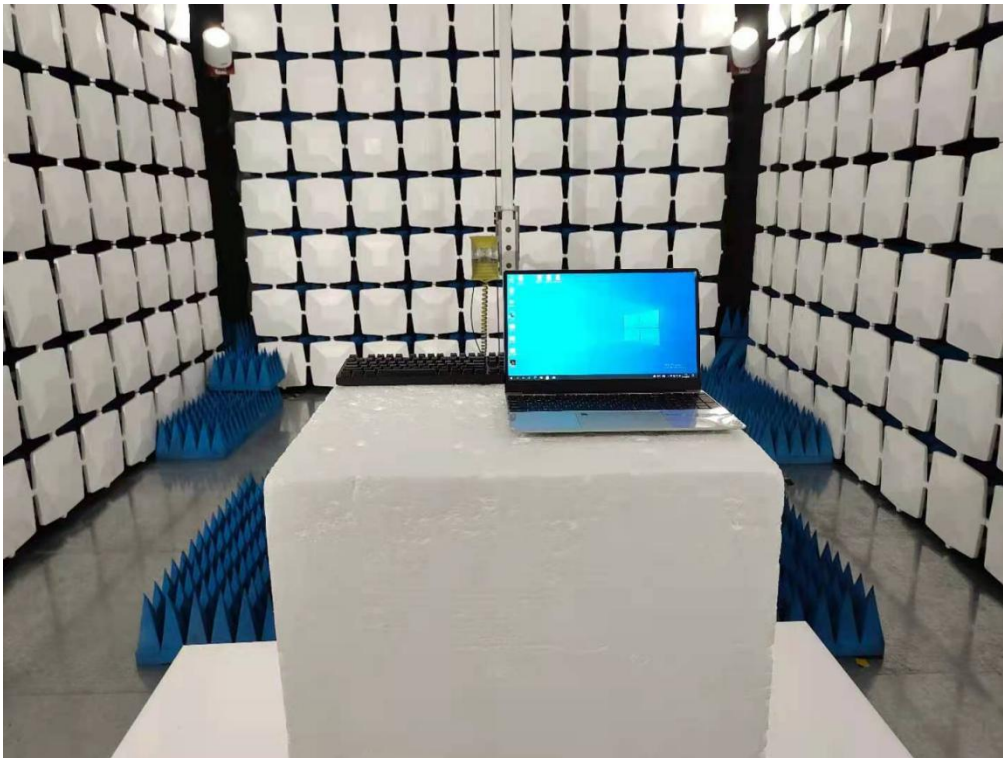
Above 1GHz for radiated emission test setup
