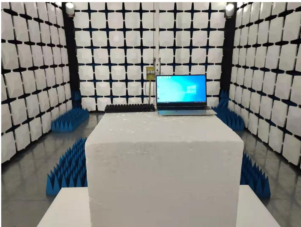
Above 1GHz for radiated emission test setup
