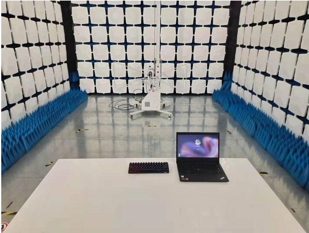
Above 1GHz for radiated emission test setup
