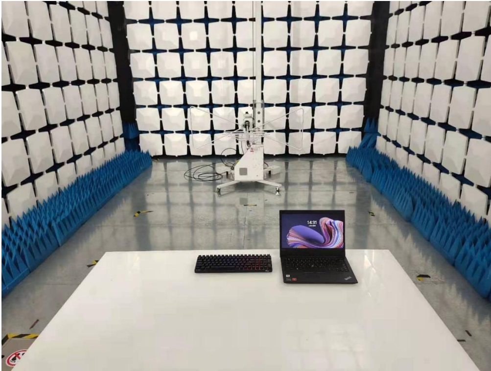
Blow 1GHz for radiated emission test setup
