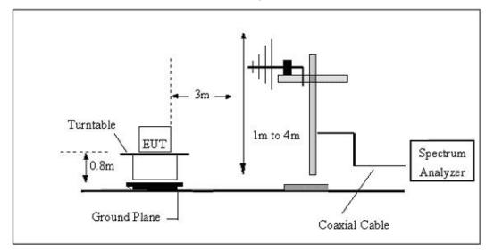
(C) Radiated Emission Test-Up Frequency Above 1GHz
