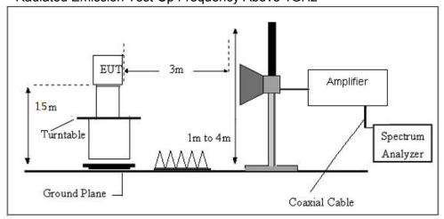
Radiated Emission Test-Up Frequency Above 1GHz
