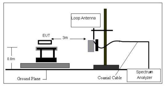
(B) Radiated Emission Test-Up Frequency 30MHz~1GHz
