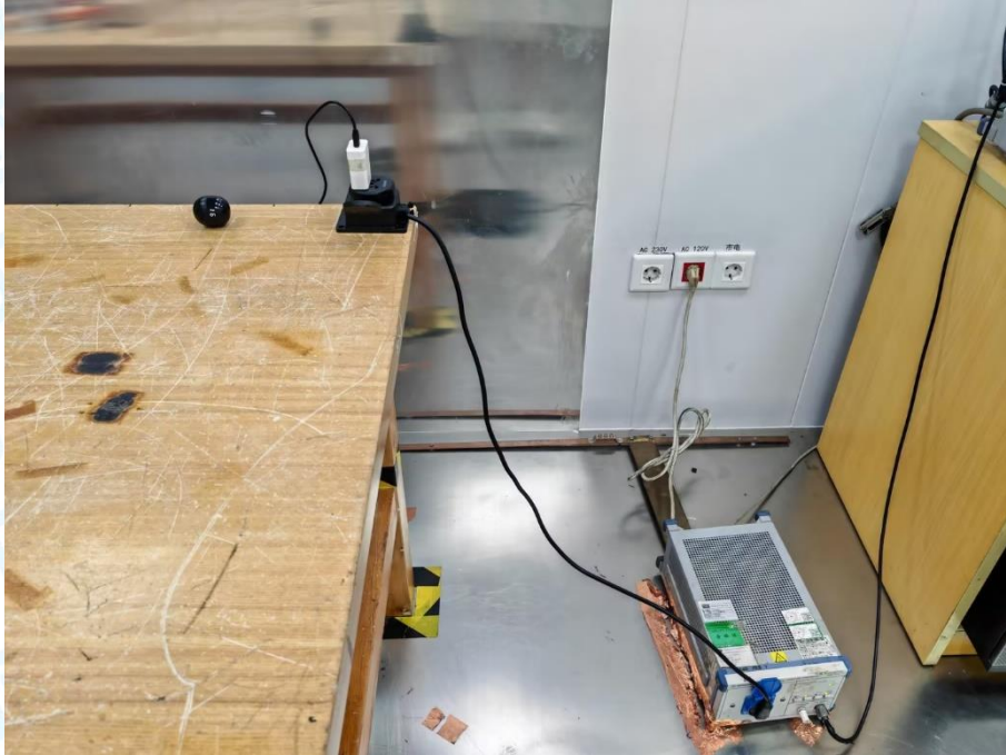
Photo of Setup for Radiated Emission (30MHz~1GHz)
