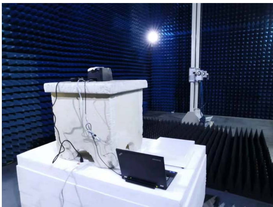
Photo of Radiated Emission Measurement 18-25GHz - Side View
