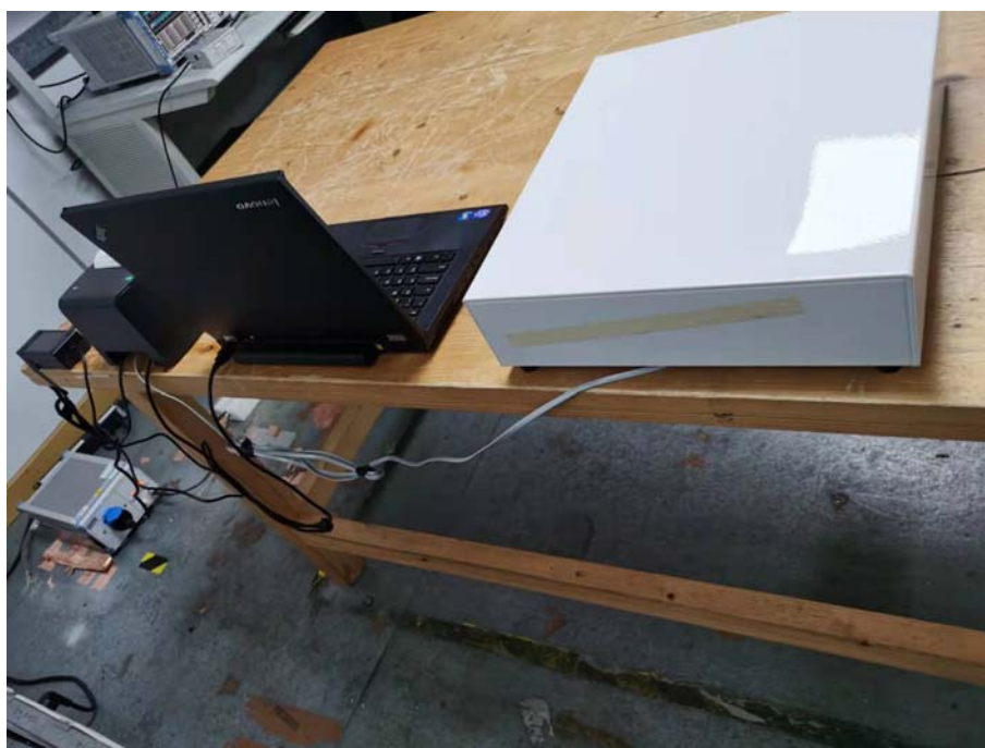
Photo of Power Line Conducted Emission Measurement - Side View
