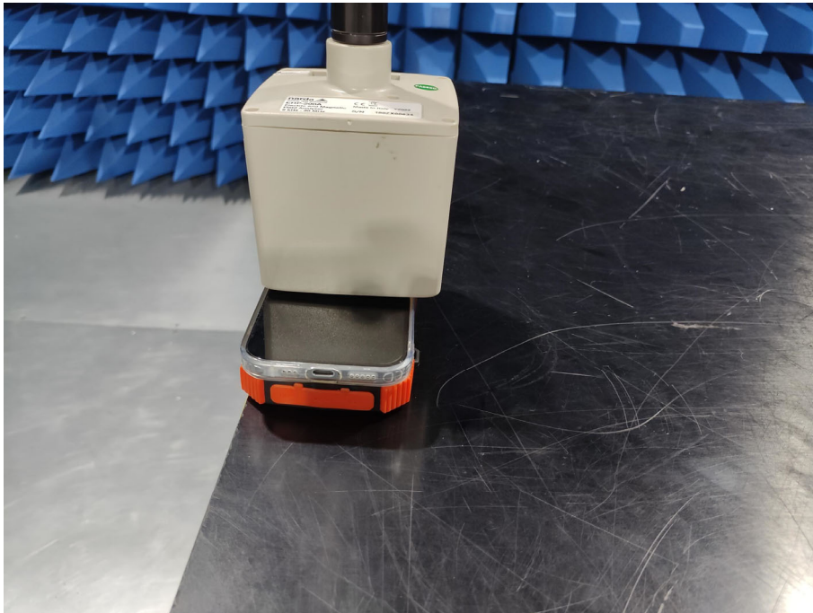
Portable exposure conditions Test Position A (0cm)
