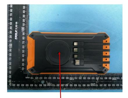
Wireless Power Bank Model: PN-W22 FCC ID: 2A4LH-PN-W22 Wireless output: 5W Input: DC 5V/3A (Max) Output: DC 5V/3A (Max)
