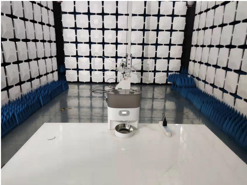
Below 1GHz for radiated emission test setup
