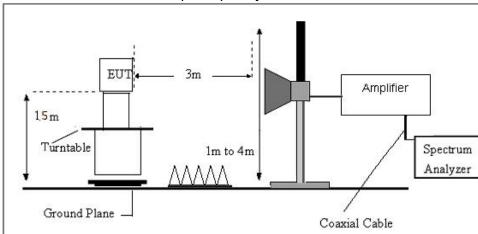
Radiated Emission Test-Up Frequency Above 1GHz
