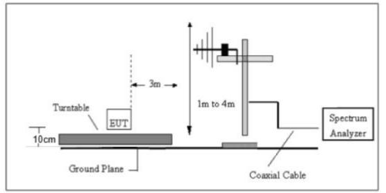
(C) Radiated Emission Test-Up Frequency Above 1GHz
