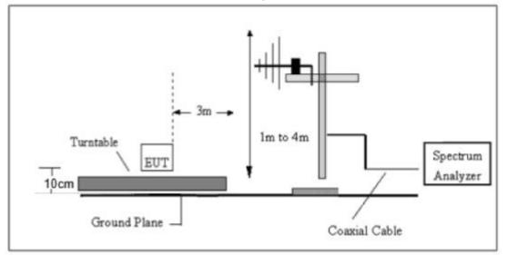
(C) Radiated Emission Test-Up Frequency Above 1GHz
