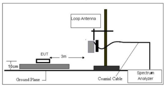
(B) Radiated Emission Test-Up Frequency 30MHz~1GHz
