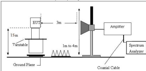
Radiated Emission Test-Up Frequency Above 1GHz
