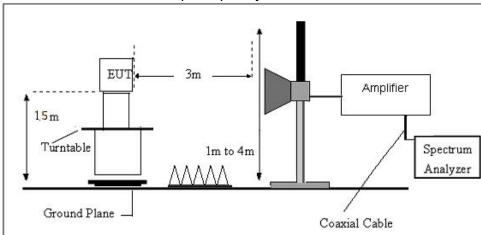
Radiated Emission Test-Up Frequency Above 1GHz
