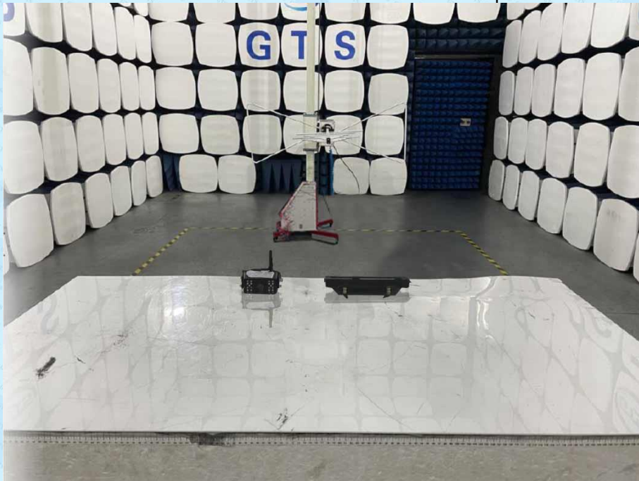
Radiated Emission Above 1GHz Test Setup
