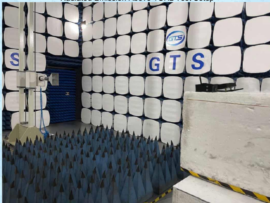
Radiated Emission Above 1GHz Test Setup
