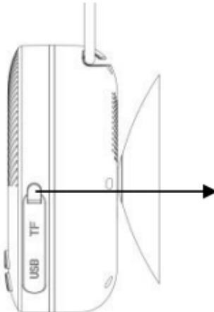
**Note:** Please tighten the Rubber Seal Cover after charging to prevent water from penetrating into the speaker.
