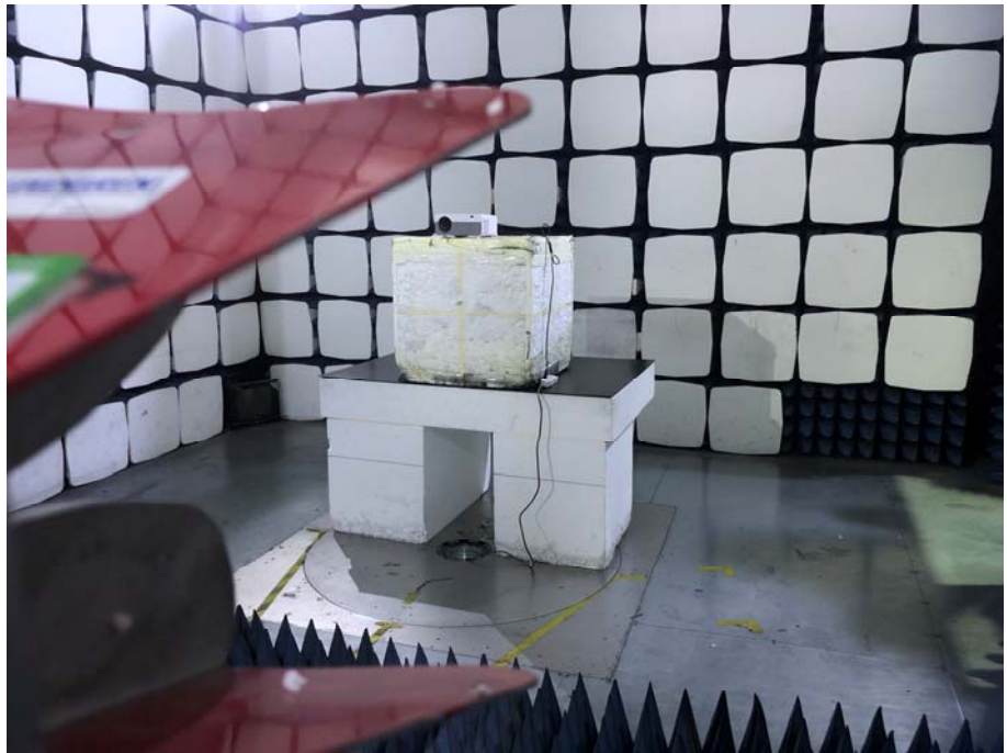
Radiation Emission Test Setup (1GHz to 18GHz)
