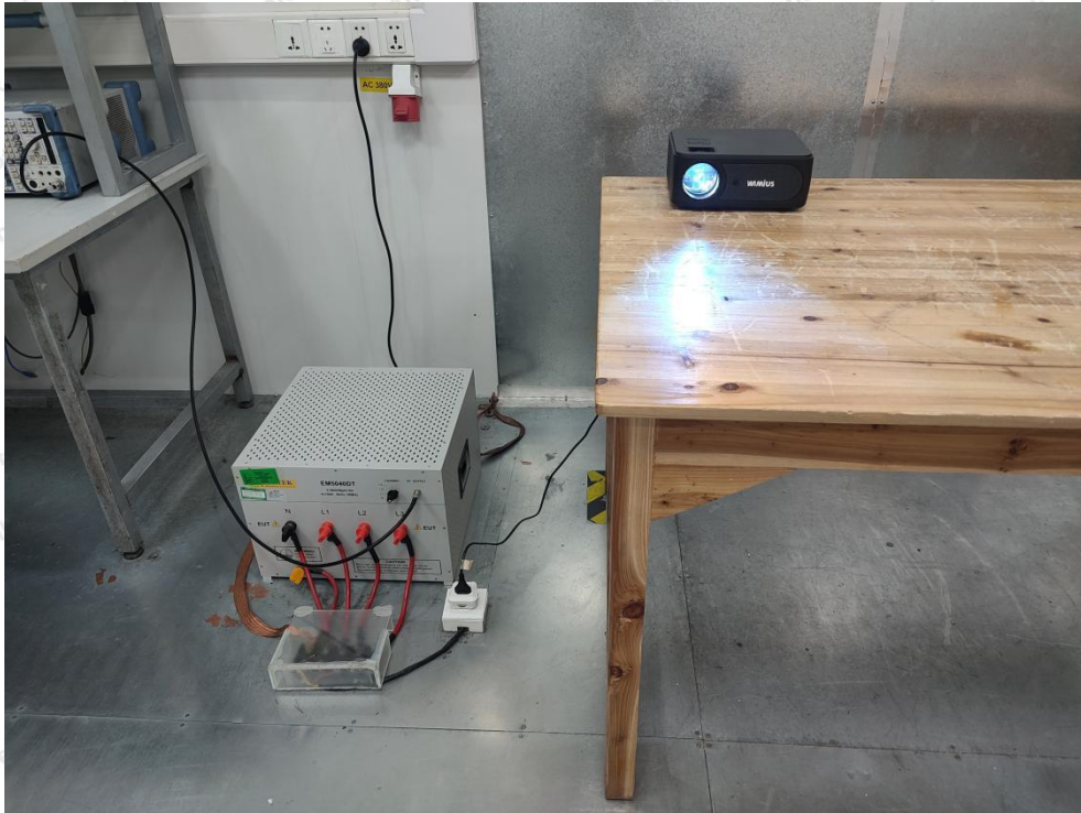
Photo of Conducted Emission Measurement
