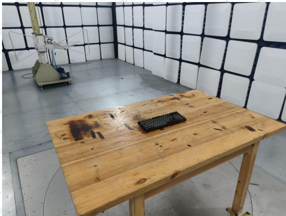
Photo of Radiation Emission Test
