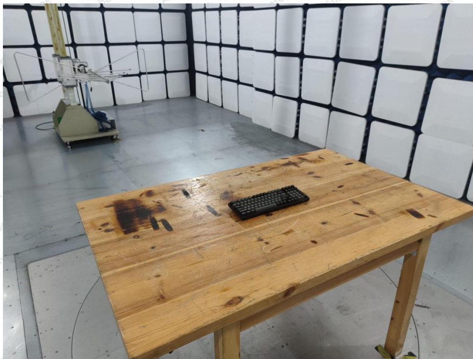
Photo of Radiation Emission Test
