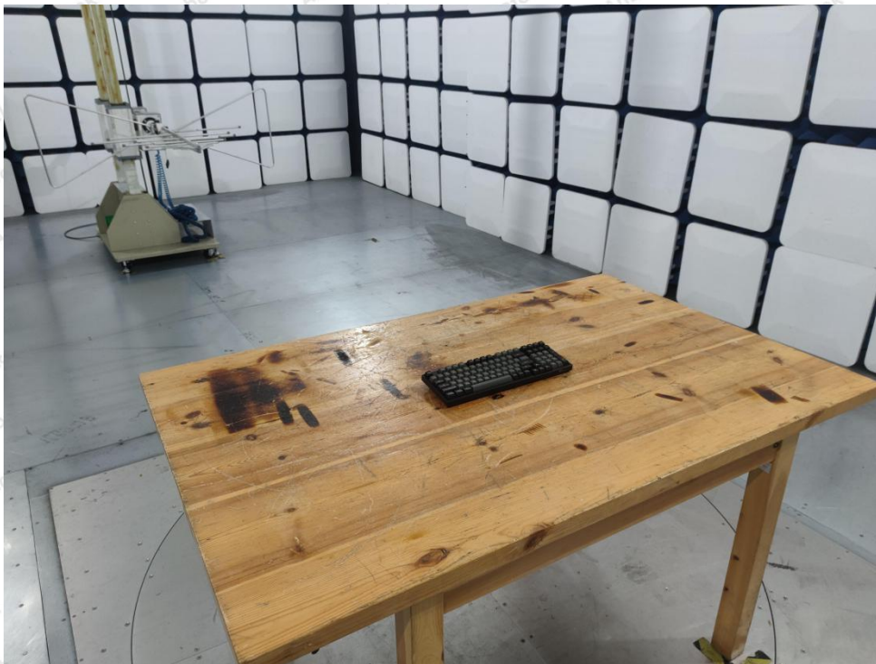
Photo of Radiation Emission Test
