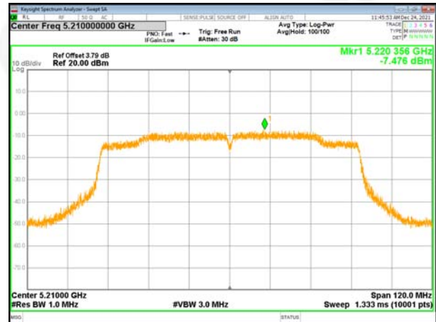
(802.11ac80) PSD plot on channel 42
