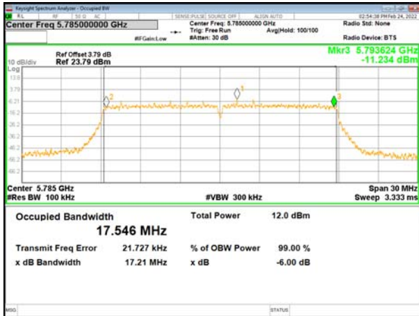
(802.11ac20) plot on channel 165
