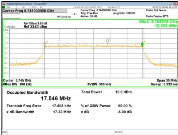
(802.11ac20) plot on channel 157
