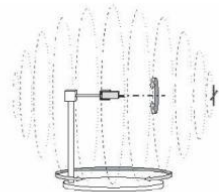
picture(2) Three-dimensional positioning device for mobile phone in darkroom
