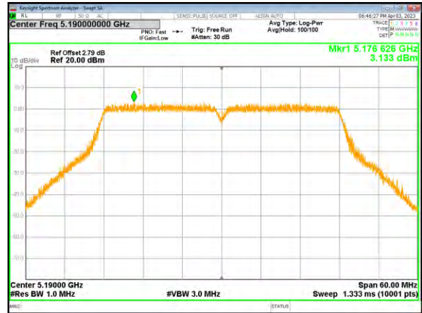
(802.11n40) PSD plot on channel 46
