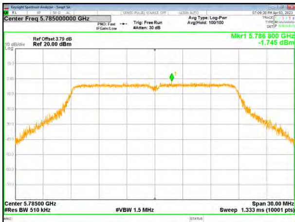
(802.11ac20) PSD plot on channel 157
