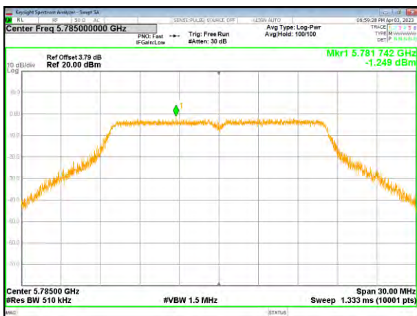
(802.11a) PSD plot on channel 157
