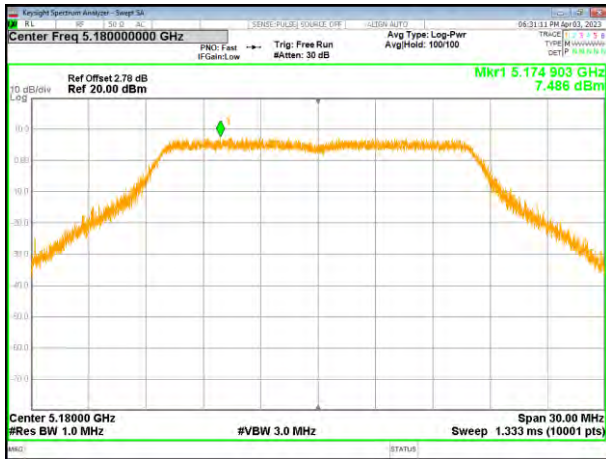
(802.11a) PSD plot on channel 40
