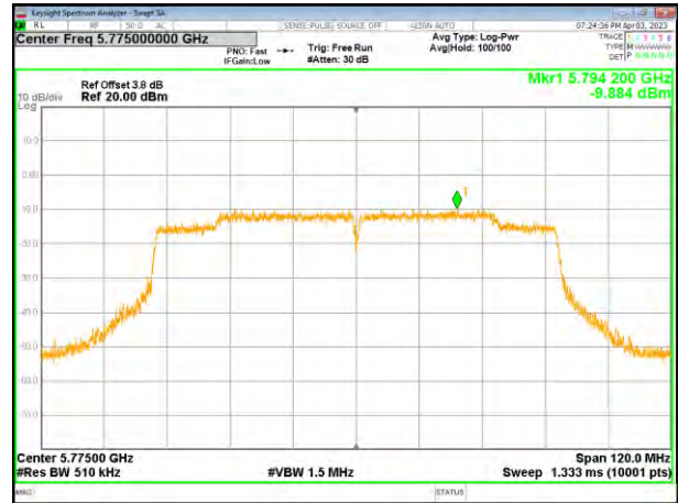
(802.11ac80) PSD plot on channel 155
