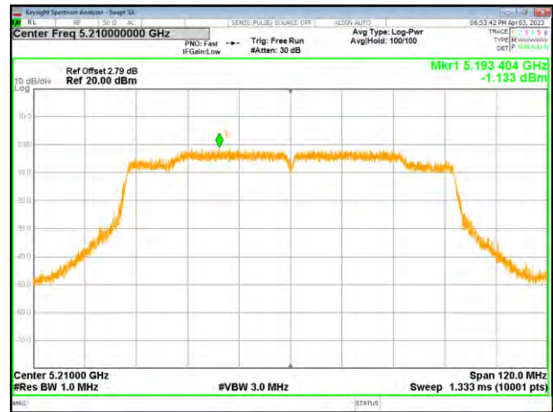
(802.11ac80) PSD plot on channel 42
