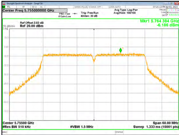
(802.11ac40) PSD plot on channel 159
