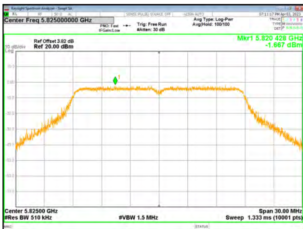
(802.11ac20) PSD plot on channel 165
