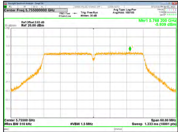
(802.11n40) PSD plot on channel 159
