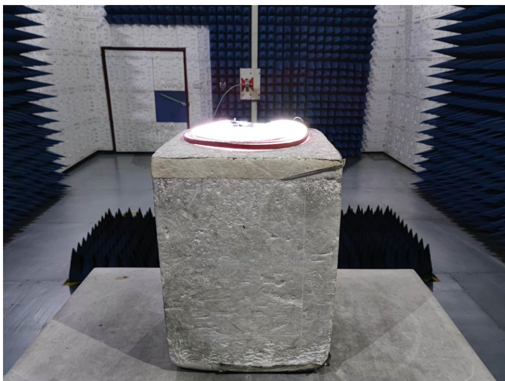
RADIATED EMISSION TEST SETUP ABOVE 1GHz
