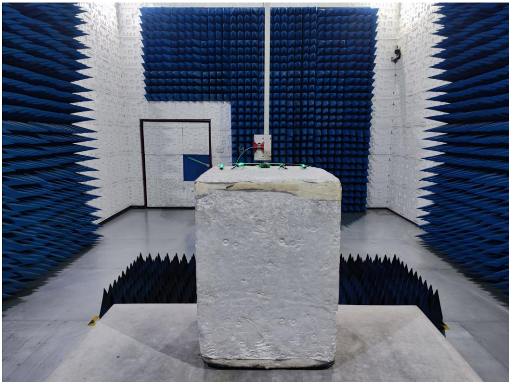
RADIATED EMISSION TEST SETUP ABOVE 1GHZ
