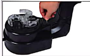
Step 2. Connect the robot head to the main engine ,then fix it with the fixed cover and screw it.
