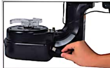
Step 3. Connect the USB line to the port of the main engine.
