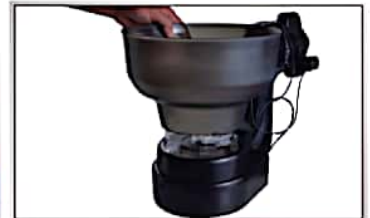
Step 4. Fix the ball storage tube to the main engine and rotate to fix it.
