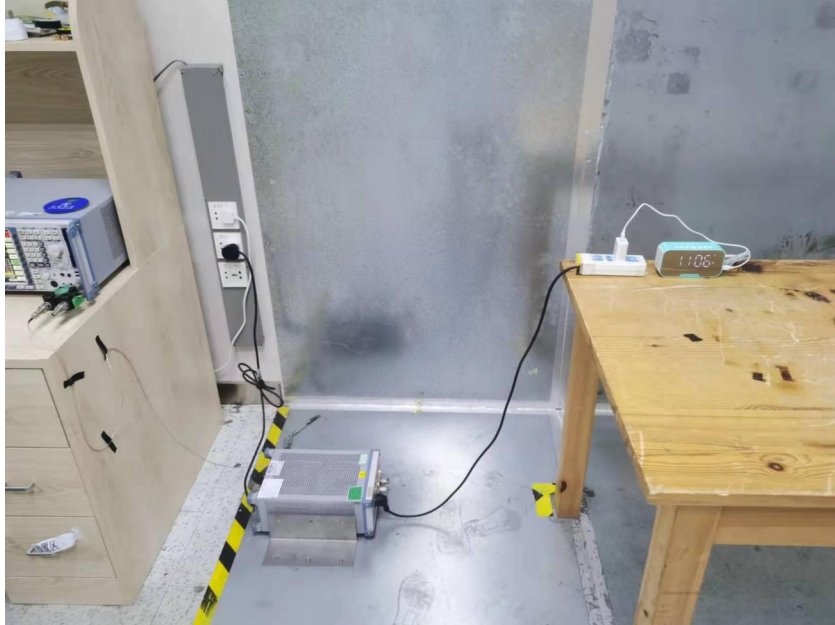
Radiated Spurious Emissions Test Frequency From 30MHz-1000MHz
