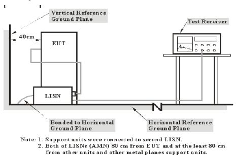
The setup of EUT is according with per ANSI C63.10-2013 measurement procedure. The specification used was with the FCC Part 15.207,RSS-Gen limits.
