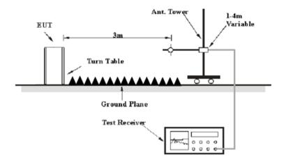
The radiated emissions were performed in the 3 meters distance, using the setup accordance with the ANSI C63.10-2013. The specification used was the FCC 15.209, and FCC 15.247,RSS-247,RSS-Gen limits.
