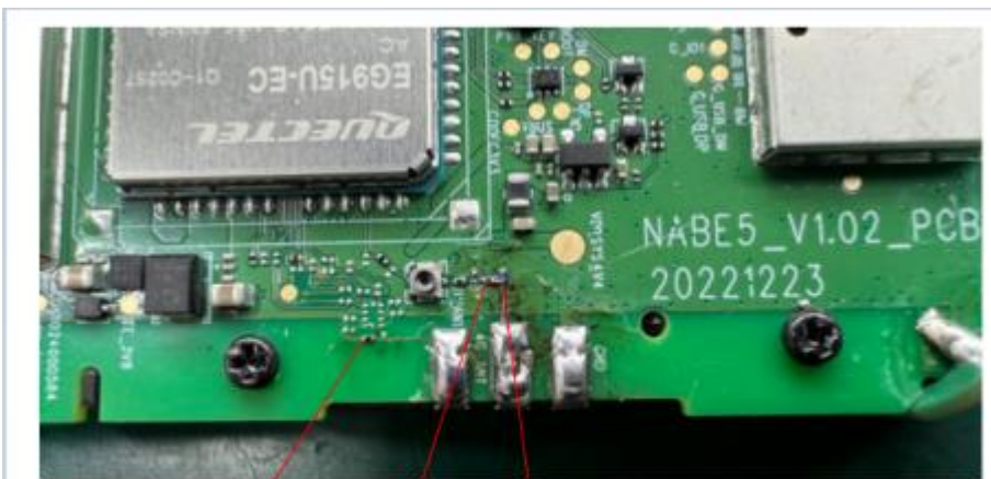
Grounding point strand 0\Omega and 12NH strand 0\Omega
