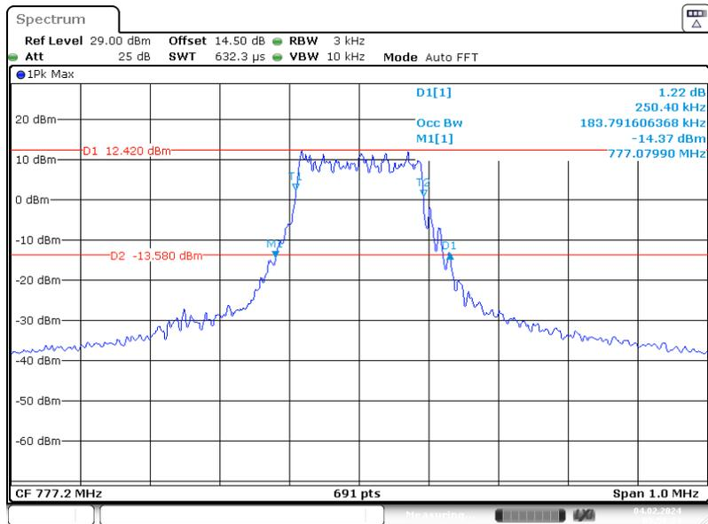
**QPSK (3.75kHz,1#0) - 99% Occupied & 26 dB Emissions Bandwidth, Middle channel**
