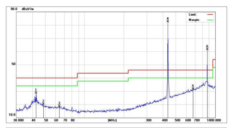
Antenna::Vertical Temperature(C):26(C) Site: LAB Limit: FCC Part 15 C 3m Radiation **Humidity(%):60%** EUT: Remote controller **Test Time:** 2022-02-18 M/N.: **KZQY24J Power Rating:** DC 3V **Test Engineer:** Mode: TX**Dyson** Note:
