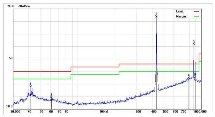
Site: LAB Antenna::Horizontal **Temperature(C):26(C)** Limit: FCC Part 15 C 3m Radiation **Humidity(%):60%** EUT: Remote controller **Test Time:** 2022-02-18 M/N.: KZQY24J **Power Rating:** DC 3V Mode: TX**Test Engineer:** Dyson Note:
