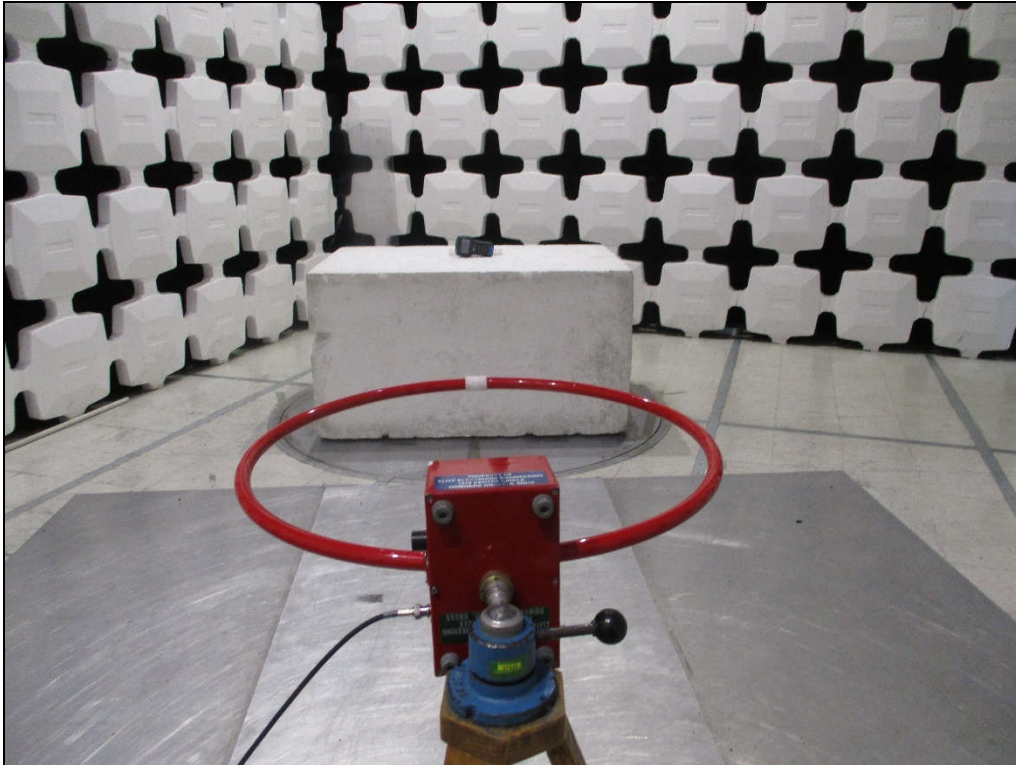
Test Setup for Radiated Emissions: 100kHz to 30MHz, Horizontal Polarization
