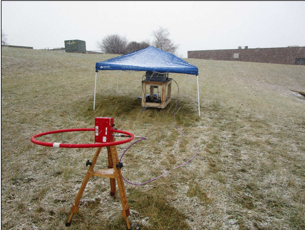
Test Setup for Radiated Spurious Emissions – 150kHz – 30MHz Z-Axis Polarization
