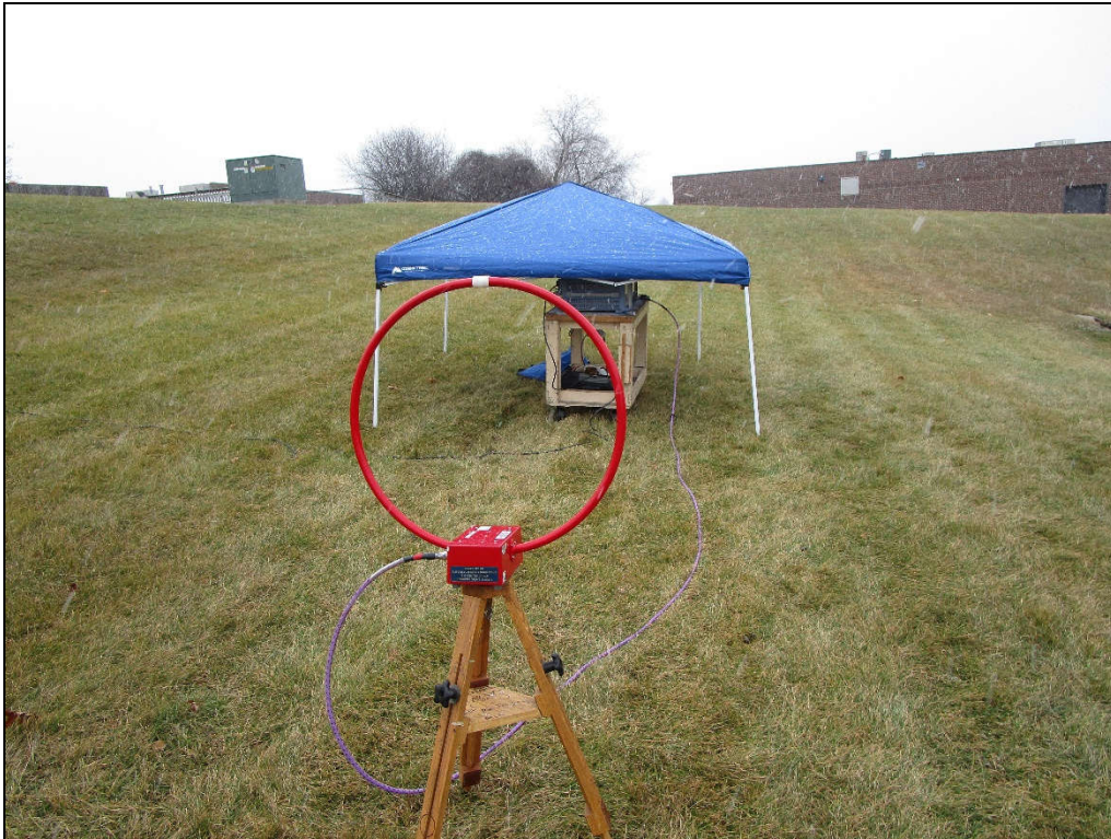
Test Setup for Radiated Spurious Emissions – 150kHz – 30MHz X-Axis Polarization
