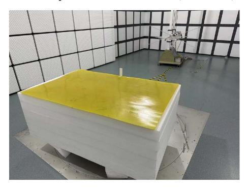
**Photo of Radiated Emission Measurement Above 1GHz**
