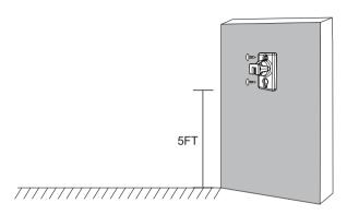
Install the transmitter mounting bracket in the desired location with the included screws.
