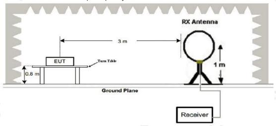
2. Radiated Emission Test-Up Frequency 30MHz~1GHz
