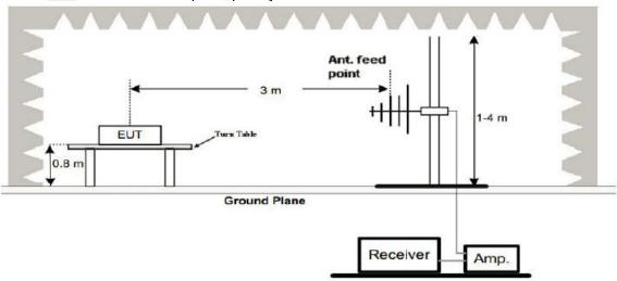
3. Radiated Emission Test-Up Frequency Above 1GHz
