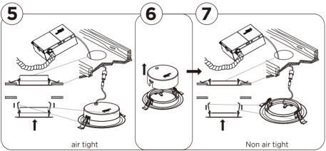
5. Use it as a air tight recessed down light, MIN height above ceiling is 2inch
