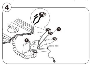
Open the connectors box cover. Feed supply wire into knockout hole using connector and make all connections inside the junction box using the EZ connectors (see picture below). Connect the 120V line wire to the black wire. Connect the neutral wire to the white wire. Connect bare copper wire to grounding terminal of the outlet box. Put on junction box cover.
