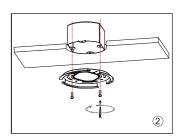
② Fix the MOUNTING BRACKET CC to junction box( excluded) with 2x32 SCREW AA.
