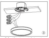
3 Pull out live wire, neutral wire and ground wire with junction box, and connect with LIGHT UNIT's live wire, neutral wire and ground wire accordingly with WIRE NUT BB.
