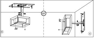
Approach LIGHT UNIT to the MOUNTING BRACKET CC, till LIGHT UNIT's center hole go through screw stem, adjust stem's length and tighten it with hex nut one, fix LIGHT UNIT with another hex nut two
