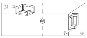
(5) Apply silicone caulking adhesive (not included) completely around the perimeter of the fixture where the back meets the mounting surface to prevent water from seeping into the junction box.
