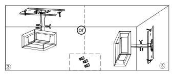
Pull out live wire, neutral wire and ground wire from junction box, connect live wire to LIGHT UNIT's black wire, connect neutral wire to LIGHT UNIT's white wire, connect ground wire to LIGHT UNIT's bare cooper wire with BB, or fix both ground wires on mounting bracket's green screw firmly.
