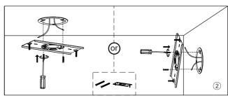
2 Use Philips screwdriver to fix MOUNTING BRACKET CC on junction box ( junction box excluded) with SCREW AA.
