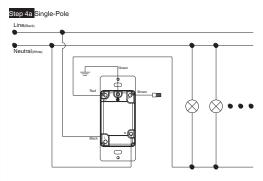
This wire is used in 3-way installations only. For single pole installations, twist with wire nut
