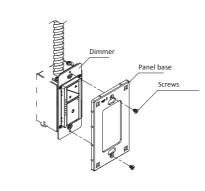
Put the panel and panel base together, press gently to make sure it is be installed firmly.
