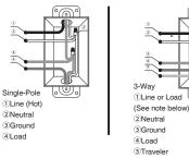
IMPORTANT: For 3-Way applications,note that one of the screw terminals from the old switch being removed will usually be a different (Black)or labeled Common (Line or Load)in both the dimmer wall box and 3-way wall box.
